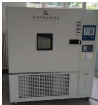
Fig. 2 GDJS-1000 damp heat test chamber
