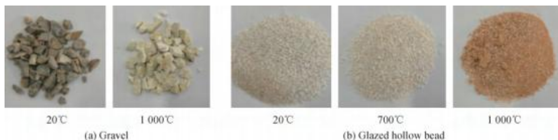
Figure 3 Appearance changes of gravel and vitrified microspheres after high temperature
