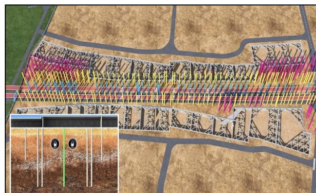
Figure 4 Construction deployment of cast-in-place piles in the central corridor
