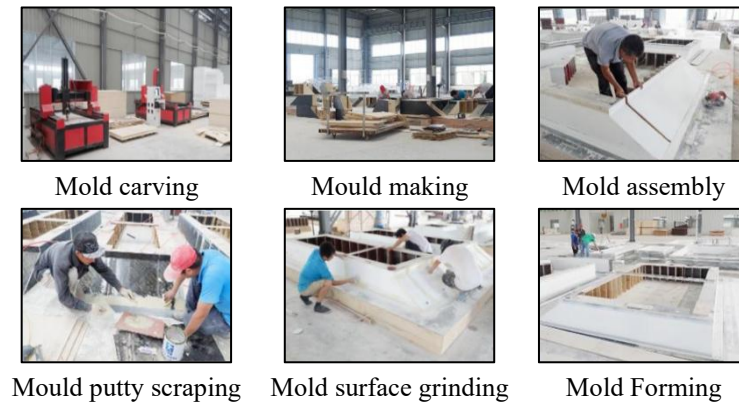
Figure 2 Flow Chart of Mold Making Process
