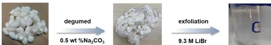
**Figure 1** Diagram for preparation process of SF aqueous solution
