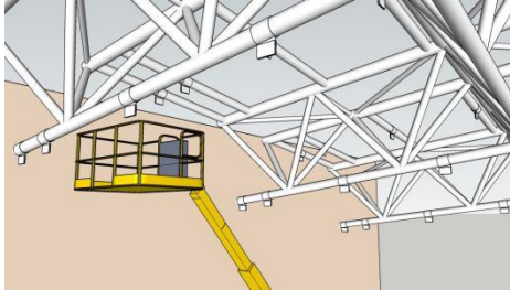
Figure 3 Installation of clamp
