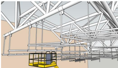
Figure 5 Installation of Horizontal Keel of Transfer Layer
