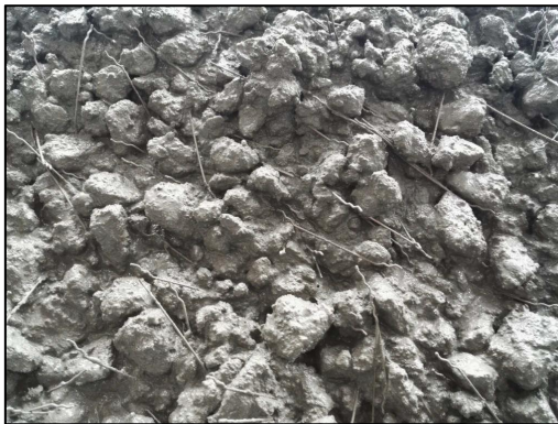
Figure 7 Steel Fiber Concrete
