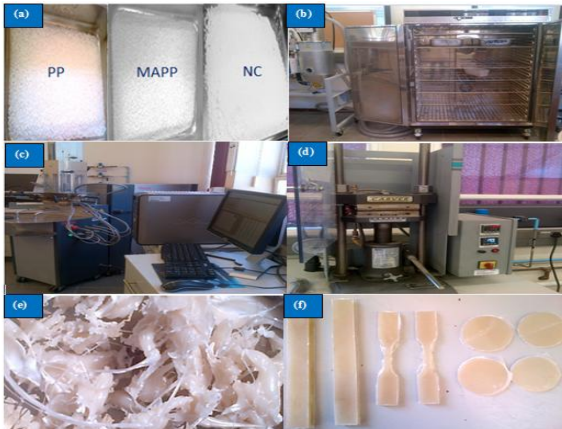
Figure 3 Image of Methodology Processes: (a) Raw Materials, (b) Oven Dryer, (c) Rheomixer, (d) Compression Mold, (e) Premixed Sample, and (f) Molded-Shaped Samples
