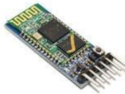
Figure 6 Wireless Communication Module
