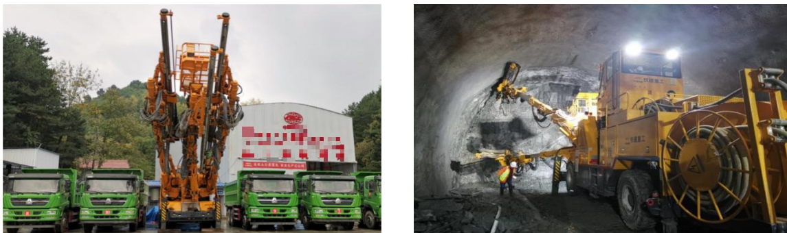
Figure 14 Three-Arm Rock Drill Dolly
