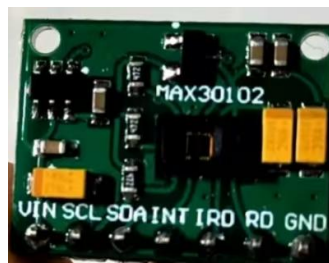
Figure 10 Physical Diagram of MAX30102 Heart Rate Oximetry Sensor Module
