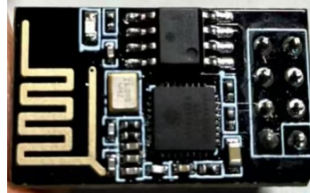
Figure 20 Physical Diagram of the ESP8266 WiFi Module
