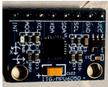
Figure 12 Physical Diagram of MPU6050 Gyroscope Module
