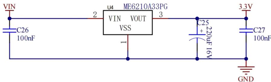
Figure 3 Schematic Diagram of 3.3V Voltage Regulator Circuit
