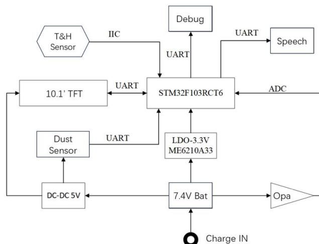
Figure 1 Overall System Block Diagram
