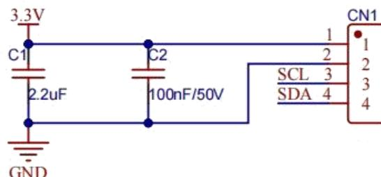
Figure 4 SHT85 Temperature and Humidity Sensor Circuit Diagram
