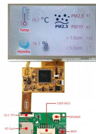
**Figure 5** Screen Connection Physical Image
