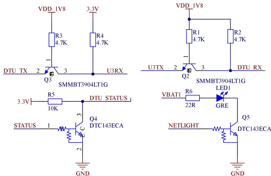
Figure 6 Design of Level Conversion Circuit in 4G Communication Circuit
