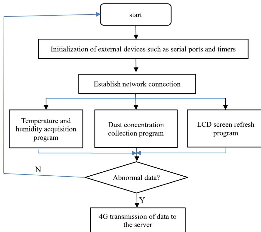
Figure 7 Overall Flowchart of System Software
