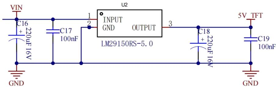
Figure 2 Schematic Diagram of 5V Voltage Regulator Circuit
