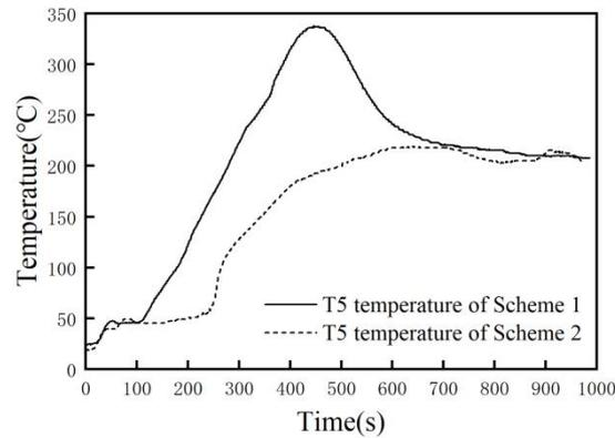
**Figure 4** T5 Temperature during Cold Start
