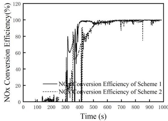
Figure 6  $NO_x$  Conversion Efficiency during Cold Start
