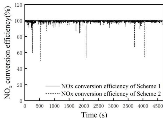
**Figure 10** NO<sub>x</sub> Conversion Efficiency during Low-load Condition
