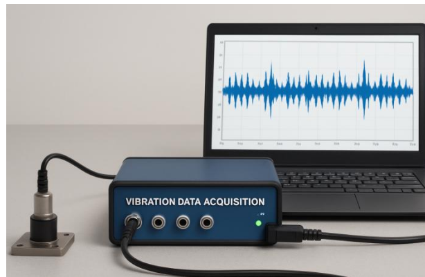
Figure 3 Vibration Signal Acquisition Equipment
