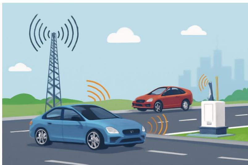
**Figure 2** C-V2X Communication between Vehicles and RSU
