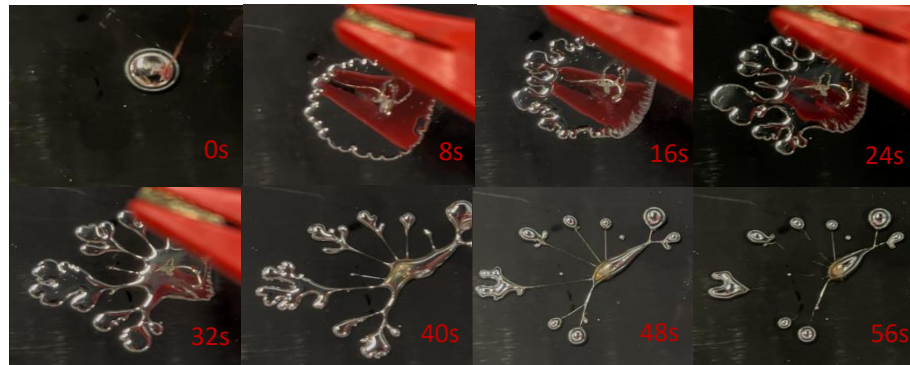
Figure 8 Morphological changes of liquid metal on graphite substrates under electric field
