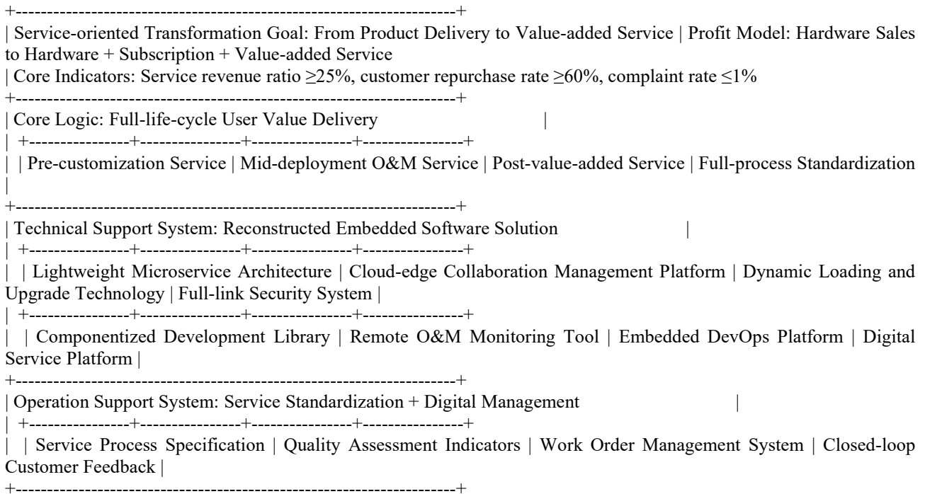
Figure 3 Relationship between Core Logic and Technical Support of Service-oriented Transformation for Embedded Software
