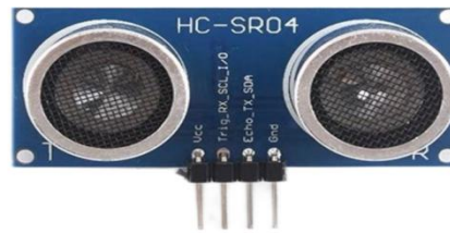
Figure 3 HC-SR04 Ultrasonic Ranging Module
