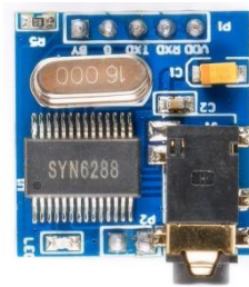
Figure 4 SYN6288 Chinese Speech Synthesis Module
