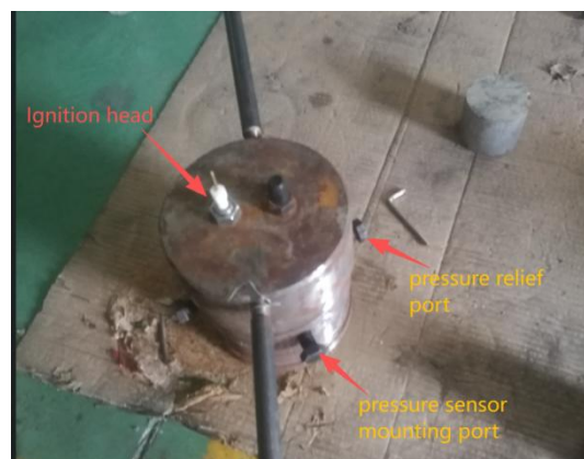
Figure 1 Actual Image of the Explosion Device
